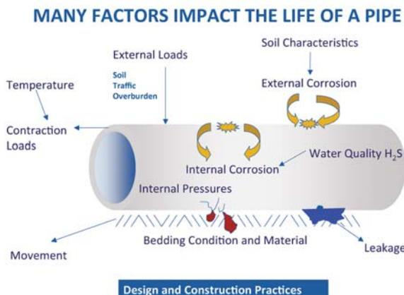
Managing buried infrastructure requires balancing the performance of the system; the associated risks; and the costs required with operational efficiency, planning requirements, affordable rate structures, security, and regulatory requirements. The decisions made to replace, or repair or rehabilitate, any pipe should be made based on the actual condition of the pipe in the system.
